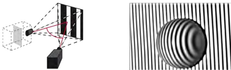
**Figure 18:** The principle behind the fringe projection technique. The projector and the camera are placed according to the triangulation angle (left). Deformation of the fringes projected onto the surface under consideration (right).
